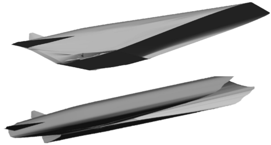
Fig. 2 Single-stage-to-orbit (SSTO) airbreathing vehicles: two-dimensional inlet and inward-turning inlet.
